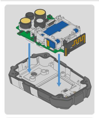
7. Install the main board into the replacement back housing.
