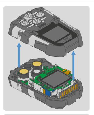
2. Remove the front housing casing and attached sensor gasket.
