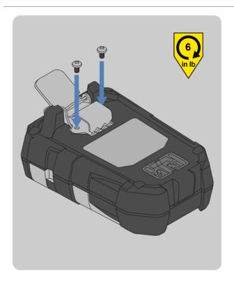
5. Install the two screws with a Phillips head #1 torque screwdriver. Torque to 6 in-lbs (0.68 N-m).
