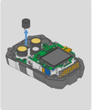
5. Remove the horn by pulling it up and out of the clear bracket.
