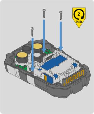
8. Install the three replacement internal screws with a Torx T6 torque screwdriver. Torque to 2 in-lbs (0.23 N-m).
