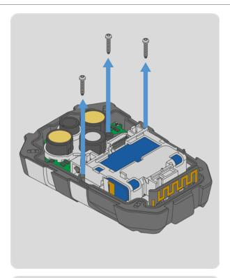
5. Remove the three internal screws with a Torx T6 torque screwdriver.
