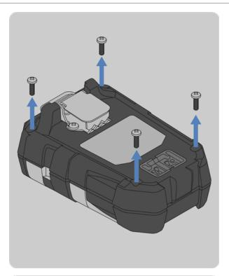
1. Remove the four external screws with a Phillips head #1 screwdriver.
