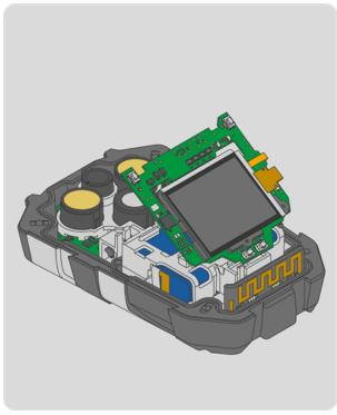
3. Remove the display PCBA and display assembly by lifting it up as shown below.
