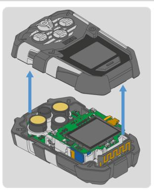
2. Remove the front housing and sensor gasket.
