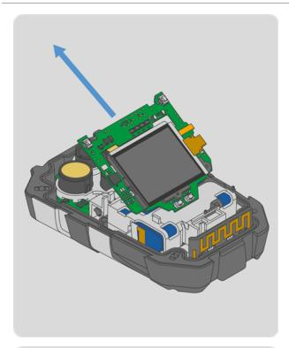
4. Lift the display PCBA and display assembly away from the main board at the angle shown. Discard according to local regulations.
