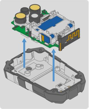
6. Lift the clear bracket and main board out of the back housing. Discard the back housing according to local regulations.
