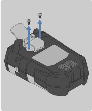
2. Remove the two screws with a Phillips head #1 torque screwdriver.
