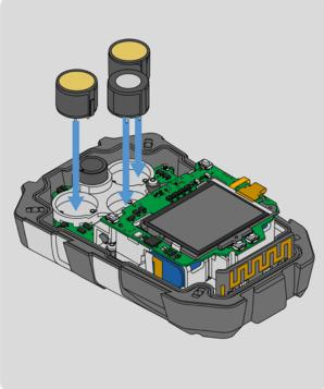
6. Install the replacement sensor(s) by pushing it down into the clear bracket.
