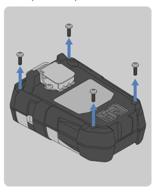
1. Remove the four external screws with a Phillips head #1 torque screwdriver.
