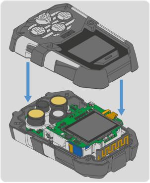
3. Install the new front housing and sensor gasket.
