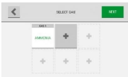
The Chillgard Ammonia monitor can only detect ammonia gas. There can be no other gas added. The 5 other slots are for different alarm settings.
