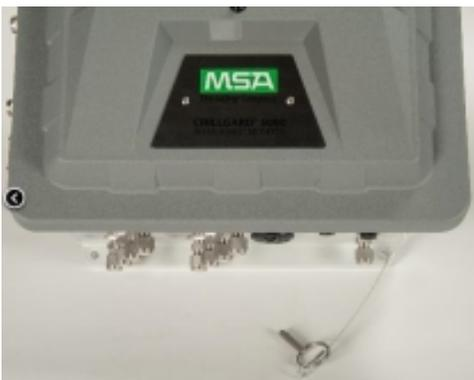
2. On the bottom of the device, remove the cap from the calibration port.
