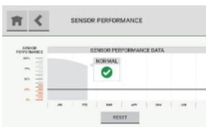
The "Sensor Performance" screen shows a graph of sensor performance over a 6-month interval. The graph is divided into quadrants. Each quadrant indicates a particular sensor status.
