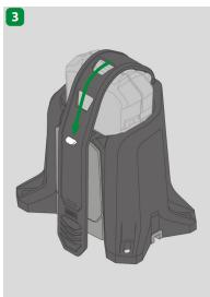
Pull the strap down over the gas detector and secure in place on the hook in the base plate. Use the slot in the strap that corresponds to the size of the gas detector.
